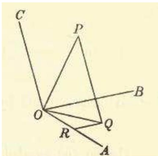
Let  $OA, OB, OC$  be the three fixed vectors,  $OP$  any other vector. From  $P$  draw  $PQ$  parallel to  $CO$ , meeting the plane  $BOA$  in  $Q$ . [There must be a definite point  $Q$ , else  $PQ$ , and therefore  $CO$ , would be parallel to  $BOA$ , a case specially excepted.] From  $Q$  draw  $QR$  parallel to  $BO$ , meeting  $OA$  in  $R$ .
